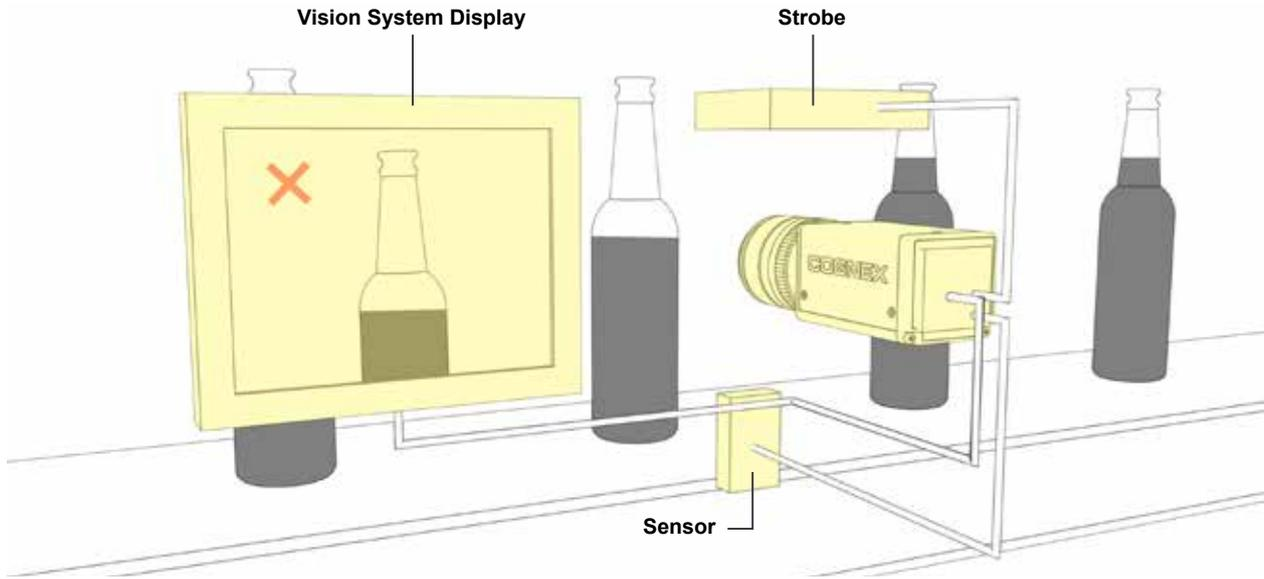
**Figure 1.** Bottle fill-level inspection example
