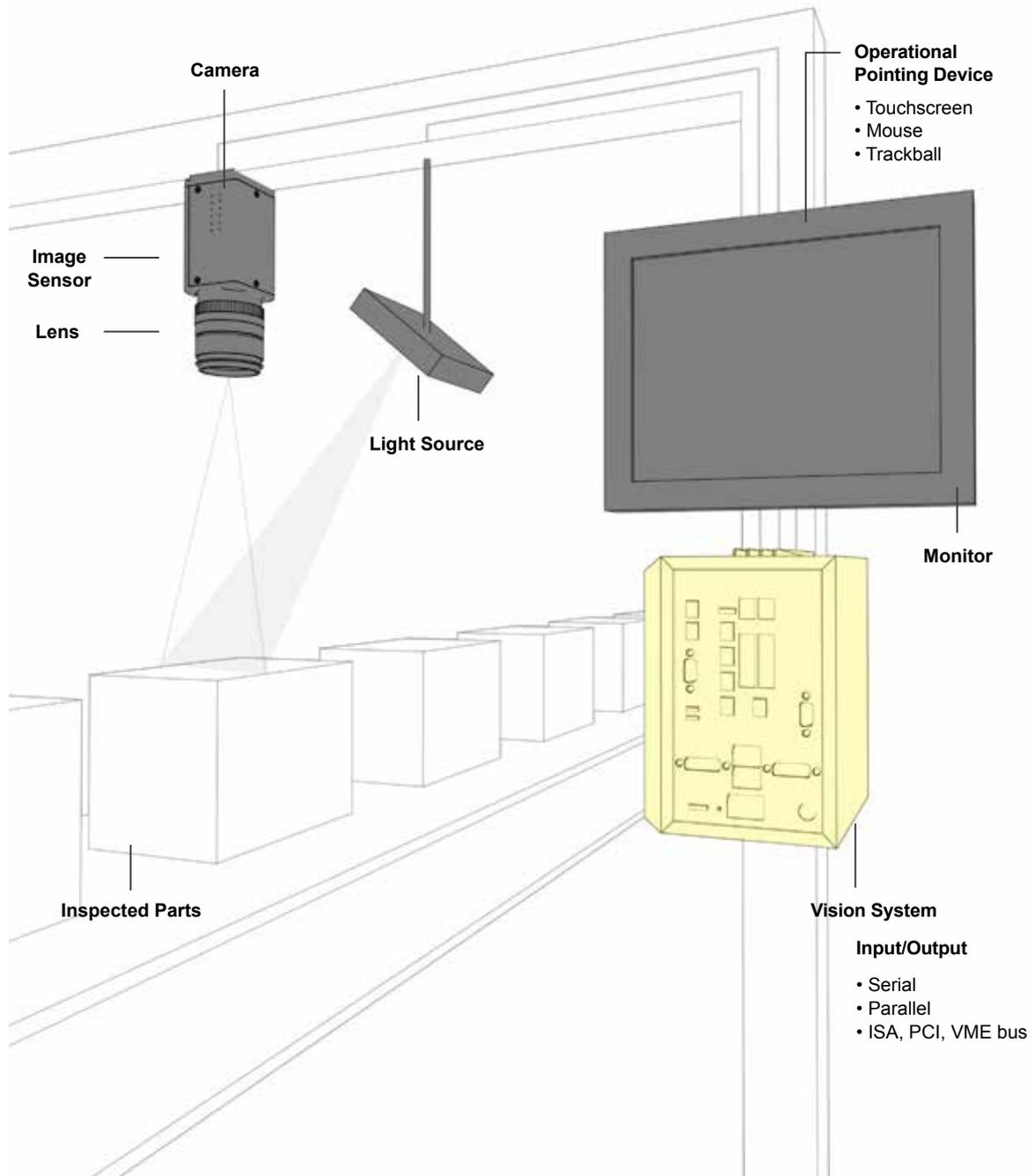
**Figure 9.** Main components of a machine vision system.
